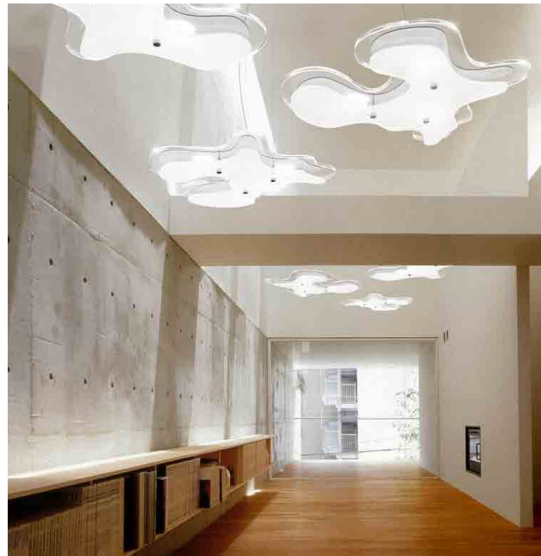
PUDDLES DIMENSION - Ø3'-3" X 3'-7" PER ELEMENT MATERIAL - ACRYLIC, ACM LIGHTING - LED
